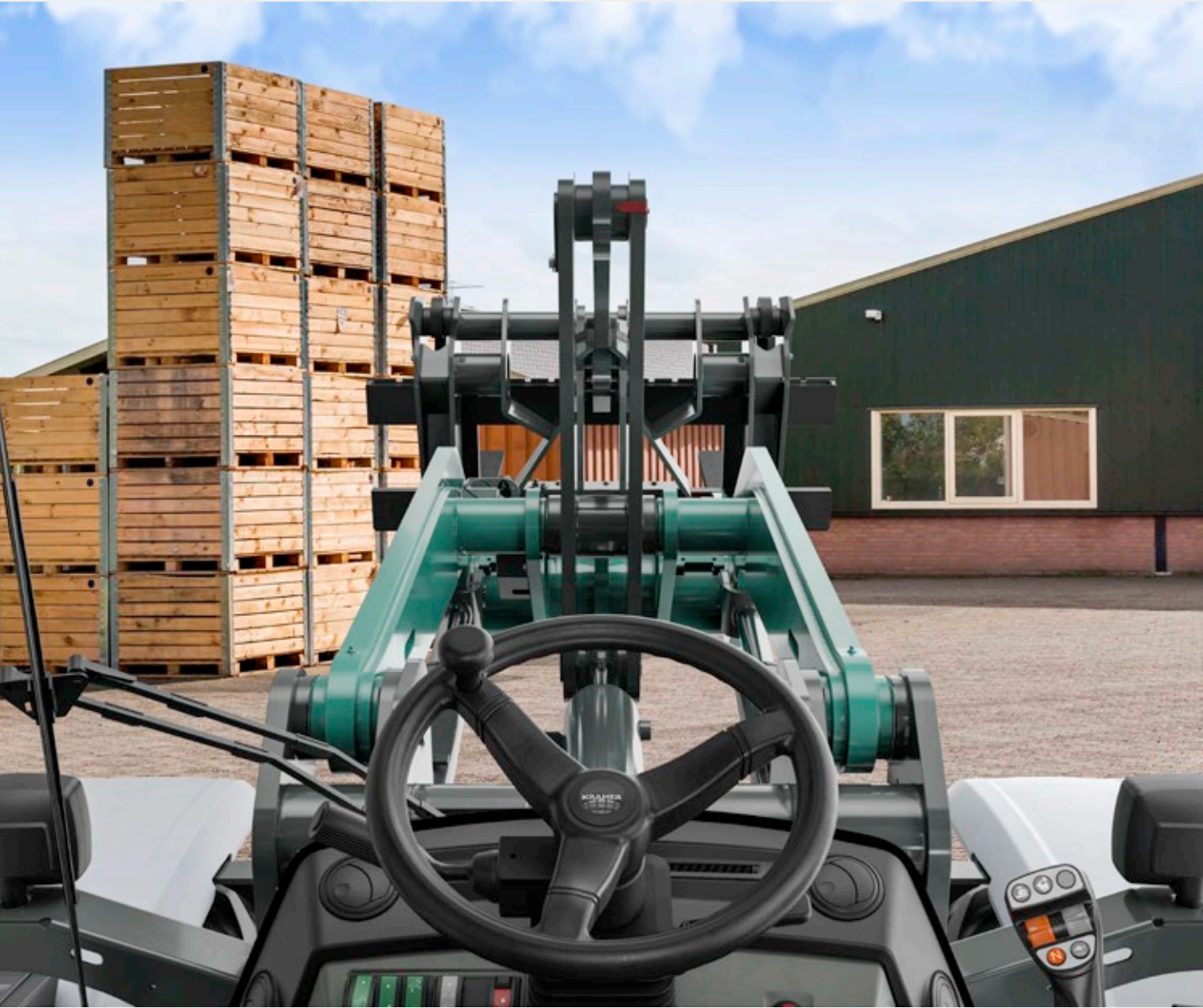
Excellent all-round visibility: a narrow cabin struts and panoramic glazing offer an optimal view on all sides.
