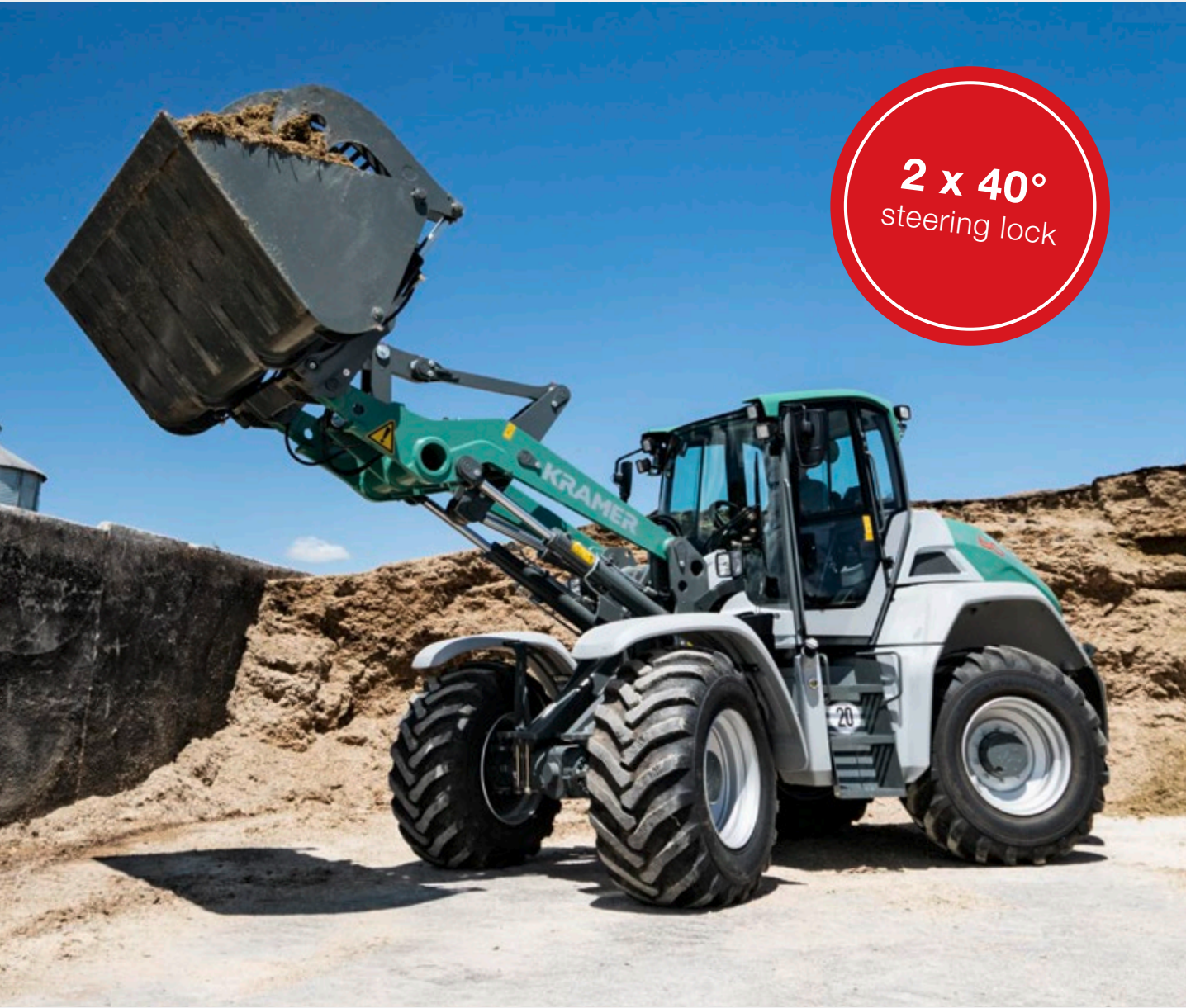
All-wheel steering is particularly manoeuvrable in tight spaces
